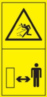
#2 - DANGER. Sharp objects could be thrown. Keep safe distance from the machine
