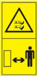
#4 - DANGER of possible shearing of limbs. Keep a safe distance from the machine while it is working.
