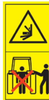
#5 - DANGER of being caught by the PTO shaft. Do not go near the rotating members of the machine while in operation.
